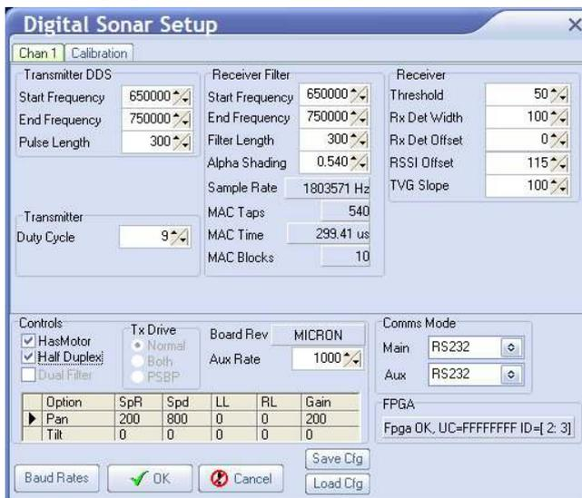
At the bottom-right of the page is the Comms Mode selection panel. Set the Aux to RS232 and click the Baud Rates button at the bottom-left of the page to open the Comms Setup window. Set the Async 1 [Head Aux/Aif Rat] baud to 9600 (for both Lo Speed and Hi Speed).
