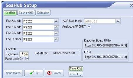
Confirm the settings and close the SeaHub Setup page. After a few seconds, the reprogramming of the unit will be complete and "Node 90, Prog Cfg Done" will be displayed in the status box. The SEAHUBNAV100 table entry will temporarily disappear from the list while the unit resets to activate the change.
