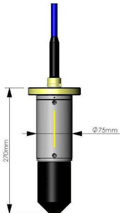
The yellow line indicates the front of transducer head. This should be positioned facing in the required forward position to ensure correct representation on the PPI display when set to “Ships Head Up”. If operating from a fixed platform/dockside this would normally be facing away from the platform/dockside and if operating from a mobile platform this would normally align with the front of the vessel.
