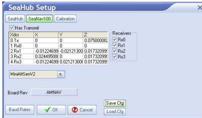
Confirm the settings and close the SeaHub Setup page. After a few seconds the reprogramming of the unit will be complete and "Node 90, Prog Cfg Done" will be displayed in the status box. The SEAHUBNAV100 entry will temporarily disappear from the list while the unit resets to activate the change.
