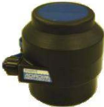
Connect the Micron Echosounder (“Main” port) to the MicronNav subsea Modem head (“Aux” port) using a Double Ended Micron Interconnect cable available from Tritech.
