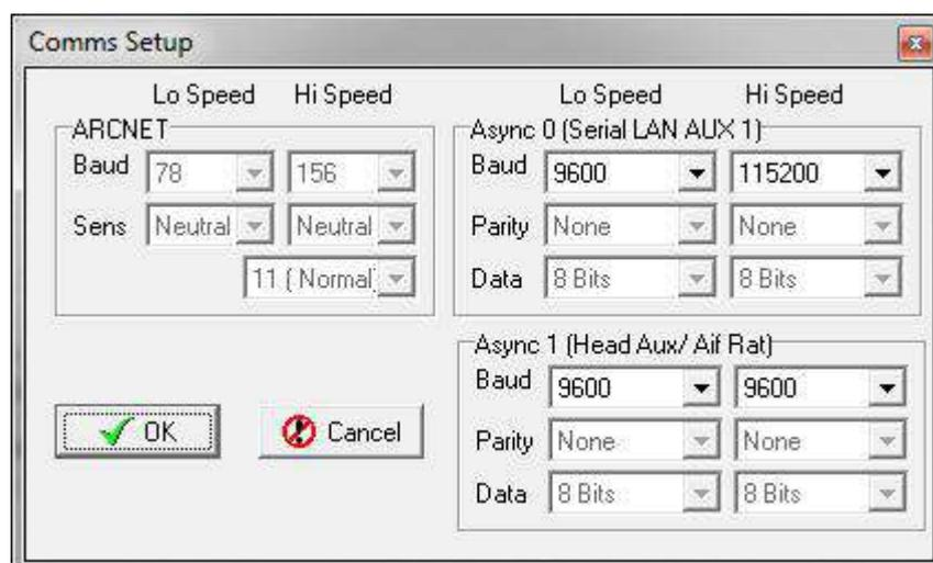
Confirm the settings and close the Comms Setup page by clicking the Ok button and then confirm the Sonar Setup and return to the Seanet Setup page by clicking the Ok button on the Digital Sonar Setup page.
