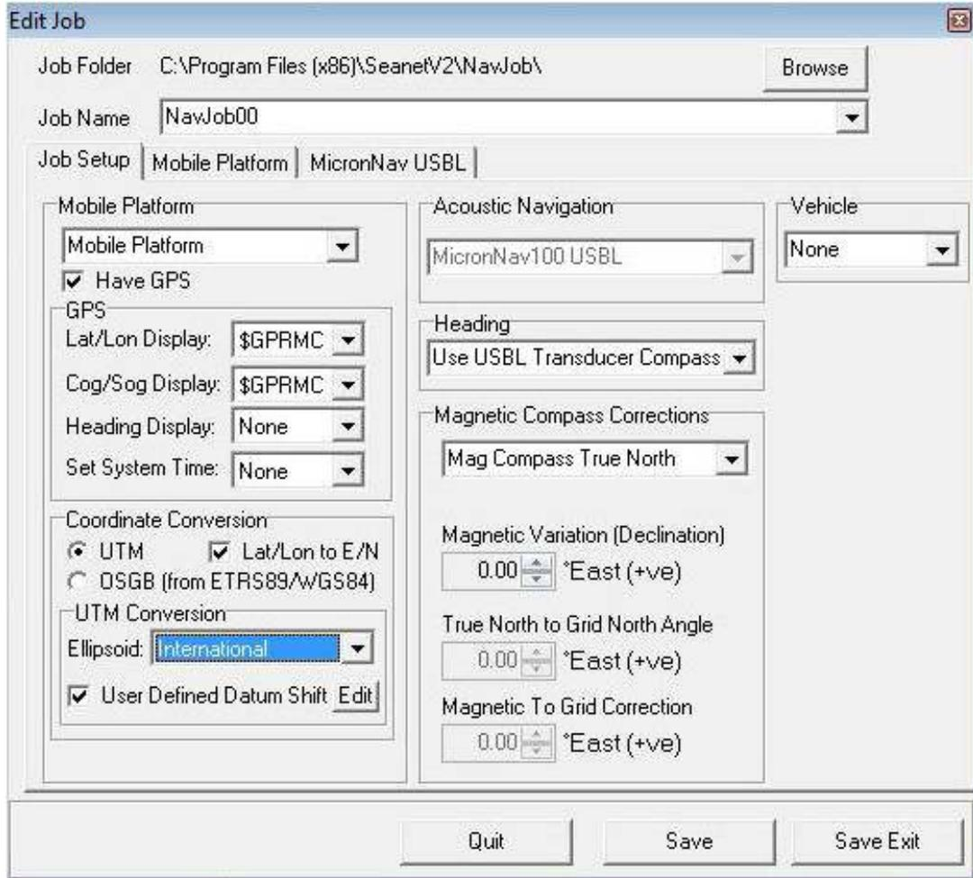
Clicking on the ‘Edit’ button to the right of the ‘User Defined Datum Shift’ tick-box, will open a ‘User Defined Geodetic Shift’ panel on top. This is used to enter the datum shift parameters.
