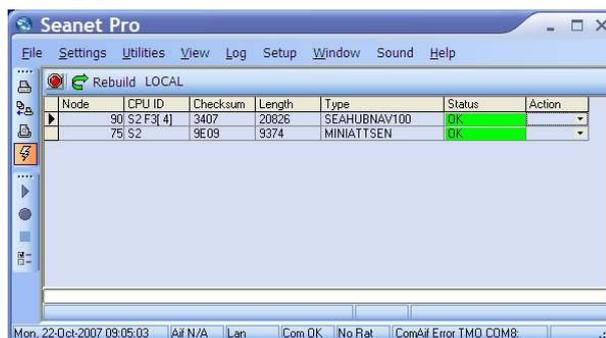
The SEAHUBNAV100 and MINIATTSEN device types should be visible in the Setup window. The MicronNav100 Hub must now be configured to communicate directly to the Transponder/Responder in order to carry out the conversion. In Seaset Setup click the Action column in the SEAHUBNAV100 row followed by Setup from the drop-down menu that appears to display the SeaHub Setup page. Set Port B to RS232.
