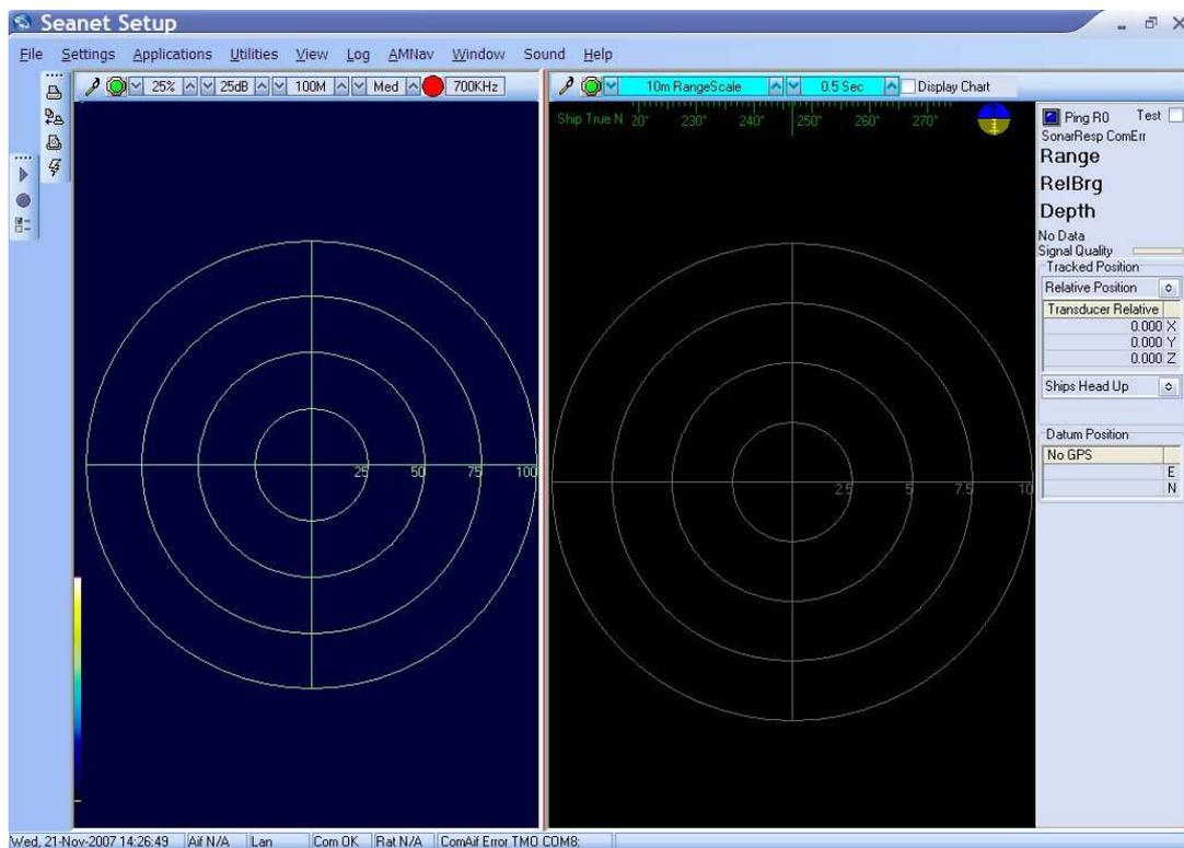
Click inside the tracking window to display the AMNav menu option in the main menu par. Select AMNav from the menu followed by Setup App from the sub-menu to open the Nav Setup page.
