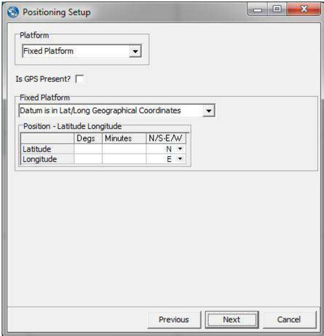
Alternatively, if there is a GPS receiver on the Fixed Platform then tick the 'Is GPS Present' check-box and select GPS message input types in the 'GPS' panel and Coordinate formats.
