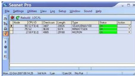
The Micron Sonar Aux port now needs to be configured for the Responder unit connection. This is done by clicking the Action arrow button in the MICRON row followed by Setup from the drop-down menu to display the Digital Sonar Setup page.
