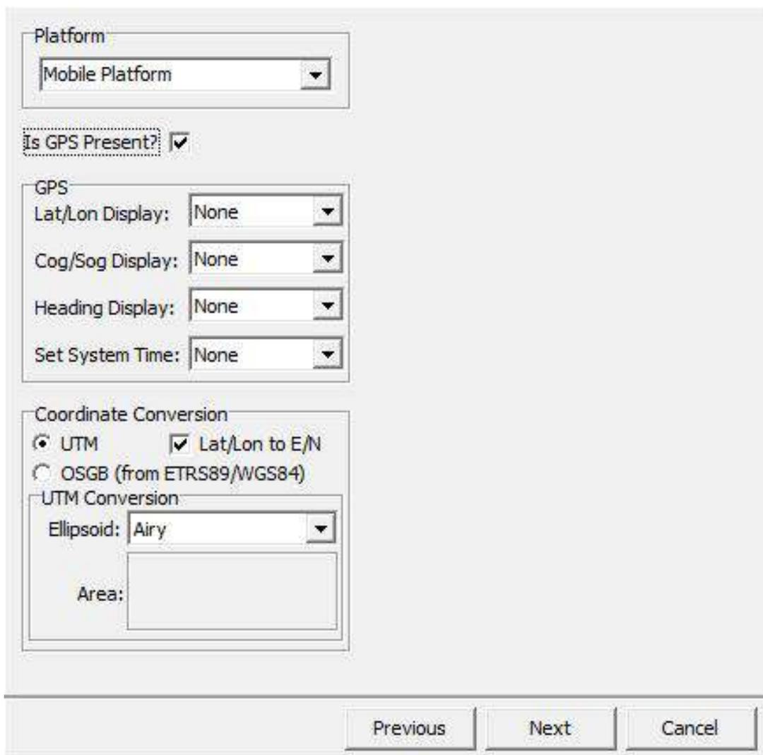
If the USBL Dunking Transducer is mounted to a Fixed Platform, then select this from the 'Platform' drop-down list. Now enter the Position co-ordinates for the Fixed Platform. This can be entered in Latitude/Longitude or UTM Grid formats.
