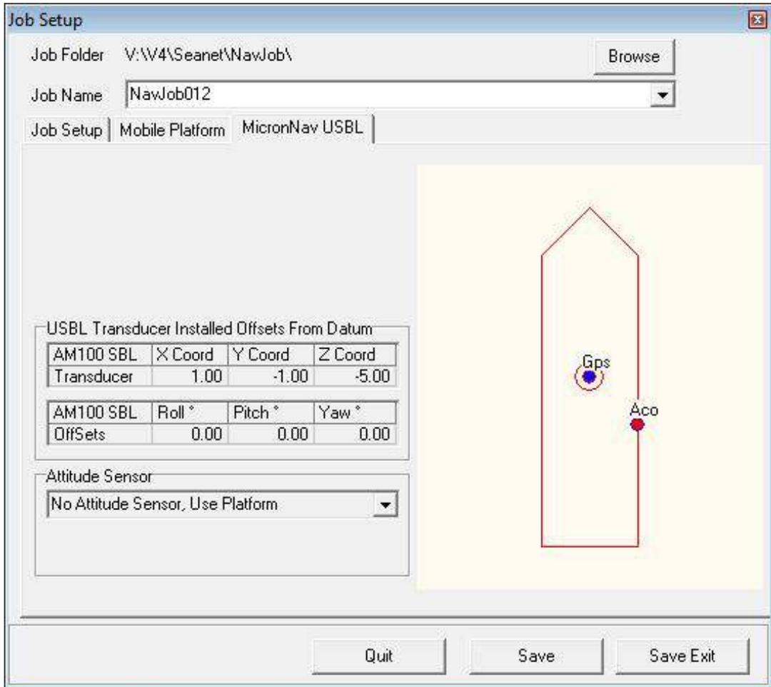
Select the source of the Pitch and Roll data, this can either be MicronNav100 Attitude Sensor (for the USBL Dunking Transducer internal sensor) or No Attitude Sensor, Use Platform if using a third party MRU sensor.
