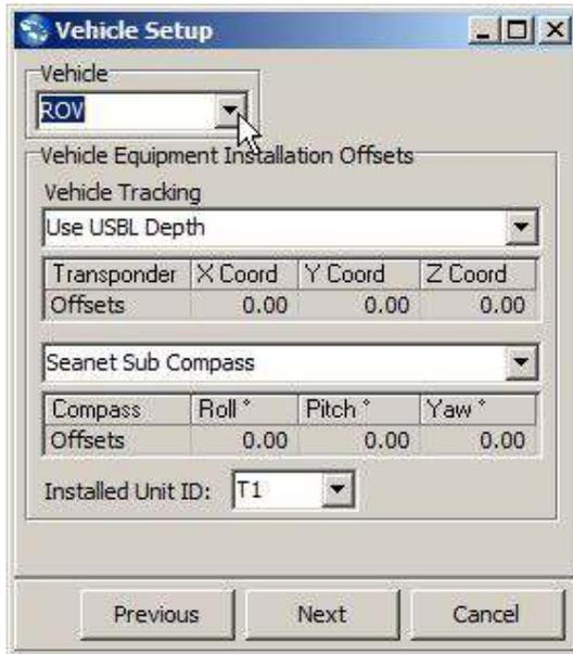
The next page of the wizard allows the user to set the Parameters for the Vessel and enter any Installation position offsets.
