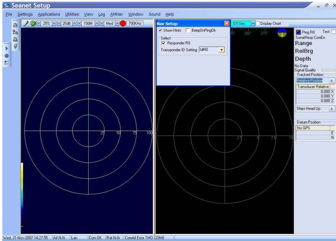
Disable the Responder R0 check-box and set Transponder ID Setting to IdM 1-16 to open the Transponder Selection options. Enable check-box T1.
