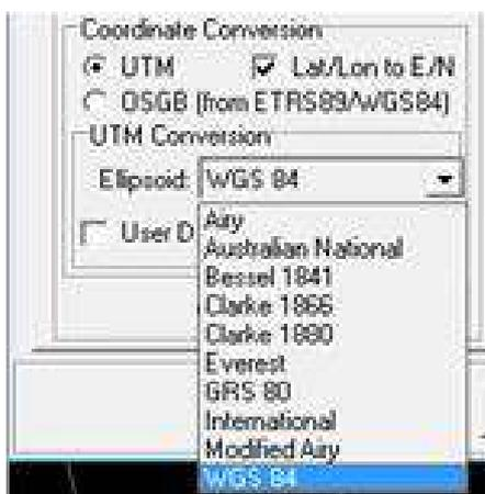
If it is necessary to display the position in Metric co-ordinates rather than Geogs, the *Lat/Lon to E/N* box must be checked and parameters set up accordingly. If using UTM then a range of ellipsoids are available.
