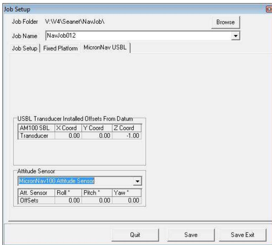
This completes the job setup for a Fixed Platform/Dockside, click on the Save and Exit button to confirm the setup and close the Job Setup window.
