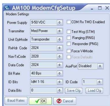
confirm the settings and close the AM100 ModemCfgSetup page. After a few seconds the reprogramming of the unit will be complete and "Node 85, Prog Cfg Done" will be displayed in the status bar.
