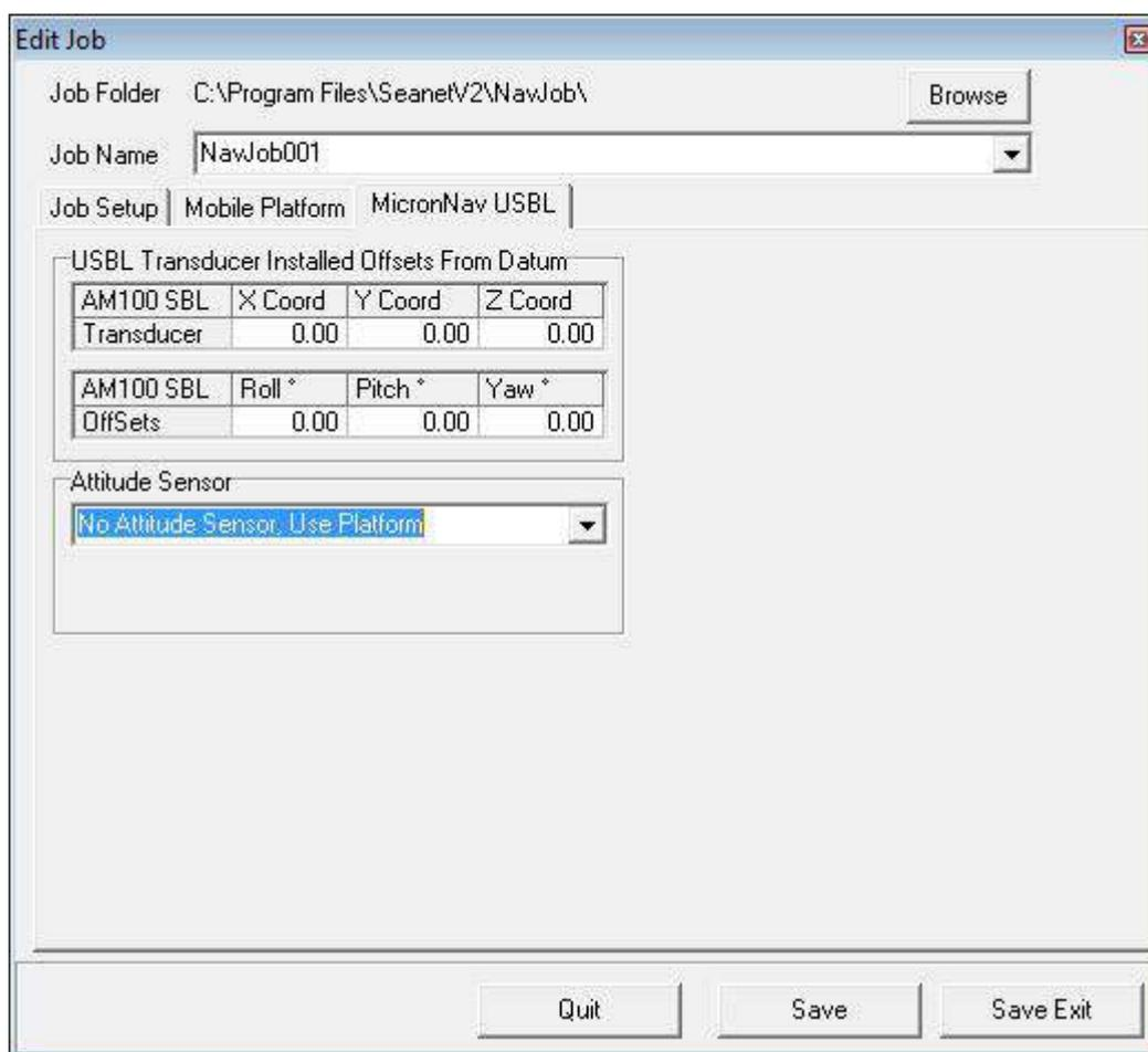
Step 3: Click on **Save Exit** to immediately update the Job and apply changes. The Integral Attitude Sensor Heading/Pitch/Roll will no longer be applied and External MRU data input(s) will now be applied instead.
