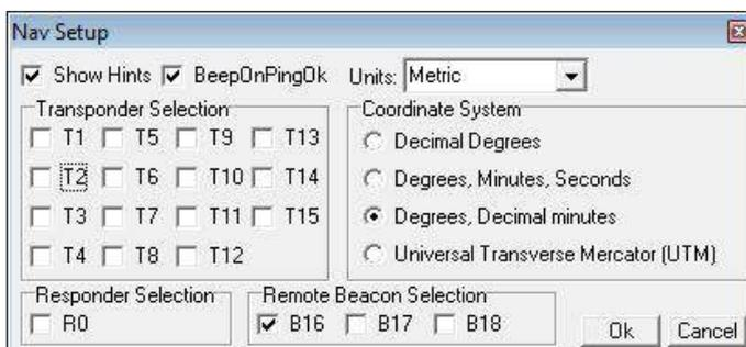
Now configure a new job in the MicronNav display. This will create a fixed or mobile datum to which the incoming remote beacon positions can be referred (to create a new job navigate to MicronNav -> Job -> Create New Job). If a job already exists it can be edited instead.
