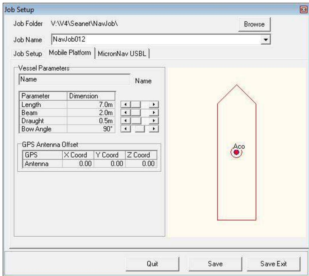
If a GPS sensor is being used enter the GPS Antenna Installation Offset measured from the transducer to the GPS antenna.
