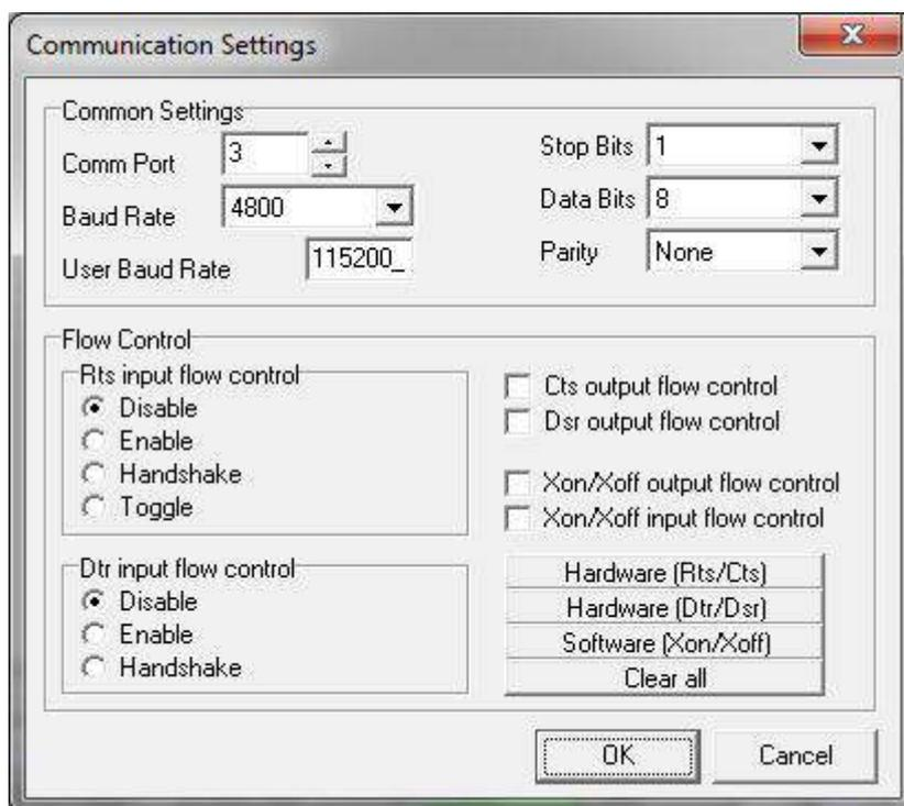
The above example shows the external Heading & Pitch/Roll sensor on COM 3 which in this case is Port A on the MicronNav100 Hub.
