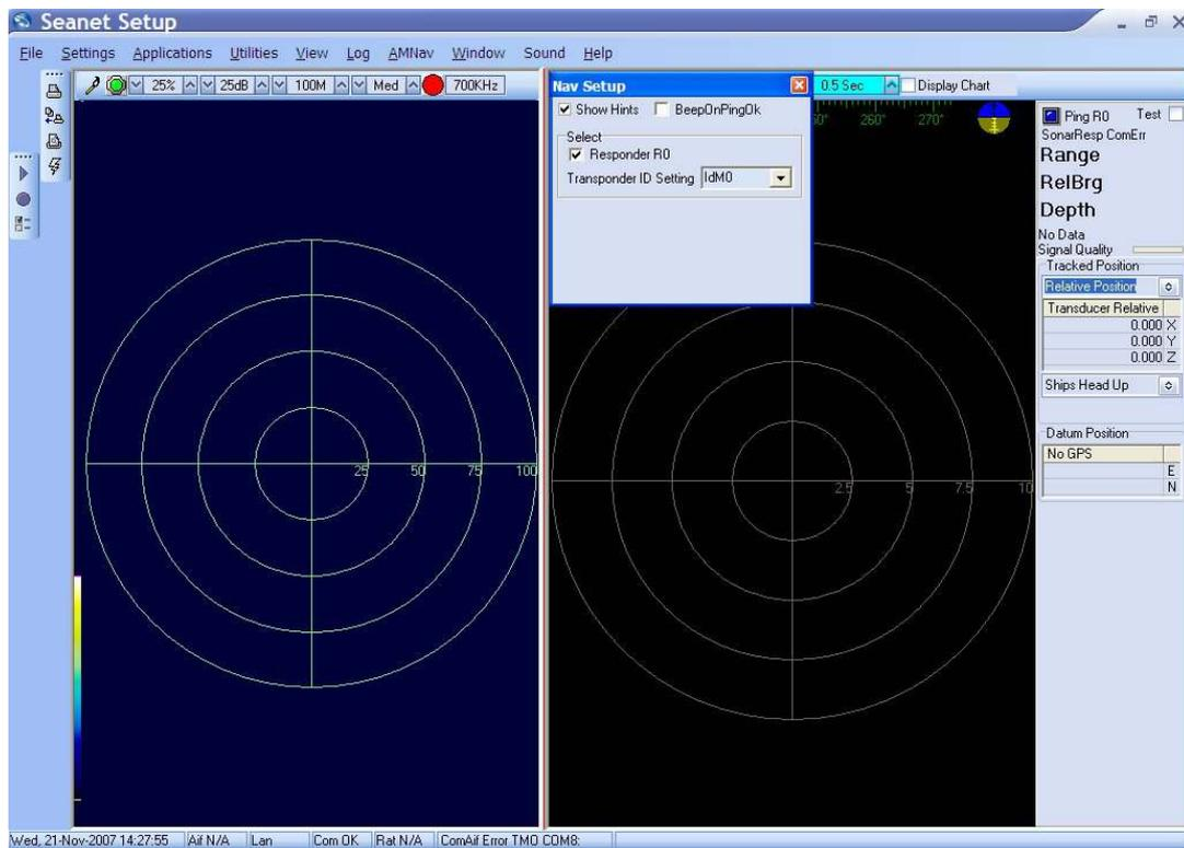
Confirm the settings and close the setup page. This completes the conversion to Responder mode. Positioning the Responder unit near the USBL Transducer head
