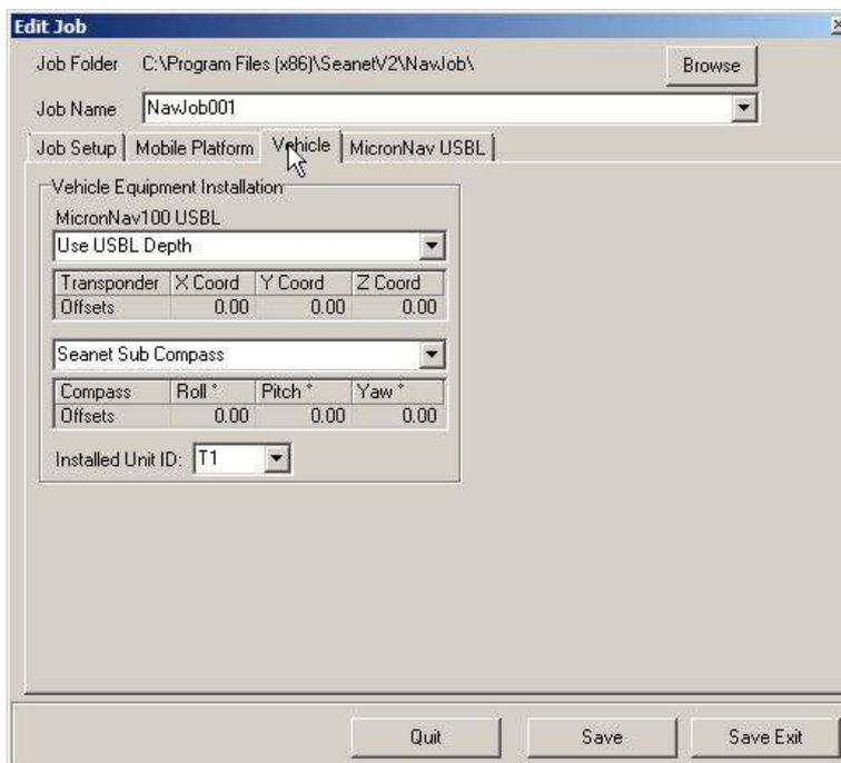
The source for the depth data for the ROV can then be configured by selecting Use USBL Depth, Use Seanet Depth Gauge or Use SK701/704 Bathy (if a SeaKing 700 Series (Bathy) is available on the system). The heading data can be selected as either No Compass or Seanet Sub Compass.
