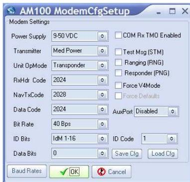
Change the Unit OpMode to Responder, ID Bits to IdM0, and enable the COM Rx TMO Enabled check-box (as shown below).
