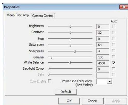
`Video Configure` is also called out from the device driver and will change according to capture device.
