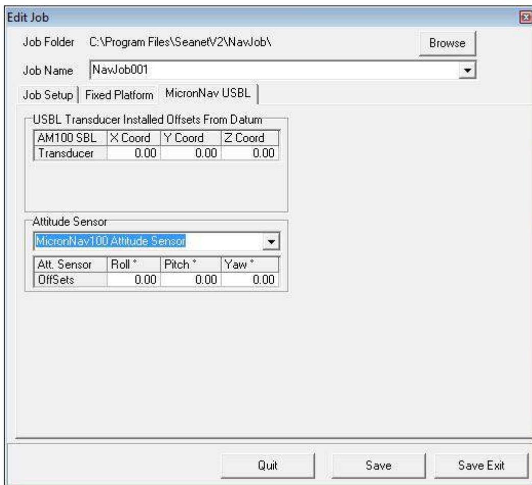
Step 3: Click on **Save Exit** to immediately update the Job and apply changes. The Integral Attitude Sensor Pitch/Roll will still be applied and the External Compass data input(s) will now be used in place of Integral Sensor Compass data.
