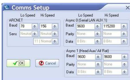
Confirm the settings and close the Comms Setup page and then confirm the Sonar Setup and return to the Seaset Setup page. Remove power from the Micron Sonar/ROV and connect the Aux port of the micron Sonar to the Main port of the Responder using an appropriate interconnect lead.
