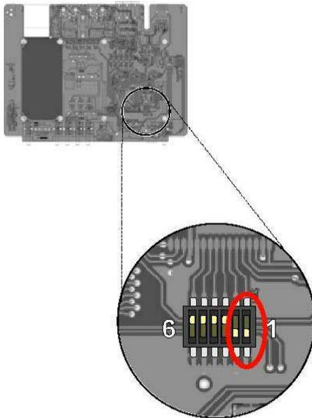
To complete the reset operation disconnect the unit from the power supply, re-open the housing as above, set switch 1 back to the OFF position and reassemble the unit. Note: If this is not done the unit will not be able to store any new settings.
