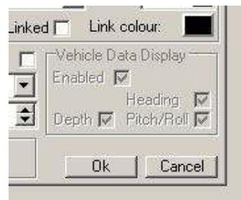
If this is the case it will be necessary to configure the ROV data by selecting Edit Job from the MicronNav -> Job menu and select ROV in the Vehicle drop down box.
