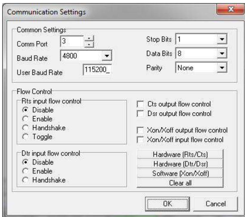
The above example shows the external Heading sensor on COM 3 which in this case is Port A on the MicronNav100 Hub.
