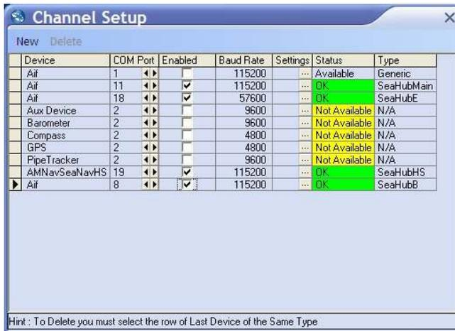
Port B should then be configured to match the Micron and ROV communications type by clicking the `Action` arrow button in the `SEAHUBNAV100` row followed by `Setup` from the drop-down menu. Set Port B Mode for RS232 or RS485 accordingly.
