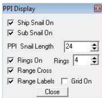
As can be seen from the captions the user can choose to display Ship Snail Trail, Sub Snail Trail, Circular rings, Range Cross, Range Labels and Grid. (In this context “Sub” refers to the tracked object or ROV) The snail trail length can be adjusted here and also the number of rings. It is suggested the user experiments with these controls to select a suitable display.
