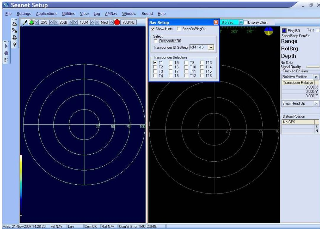
Disable the Transponder T1 check-box and set Transponder ID Setting to IdM0 which will close the Transponder Selection options. Finally enable the check-box Responder R0 (as shown below).
