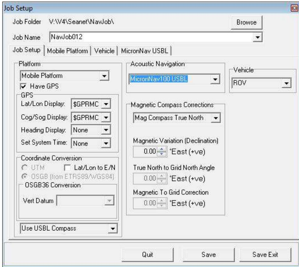
4. In the 'Coordinate Conversion' panel below that, configure this according to how position data should be displayed on-screen (and sent remotely). This can be in either Lat/Lon or Easting/Northing format. In E/N format, a UTM or OSGB projection can be performed with several Ellipsoids available for selection (with the UTM conversion).
