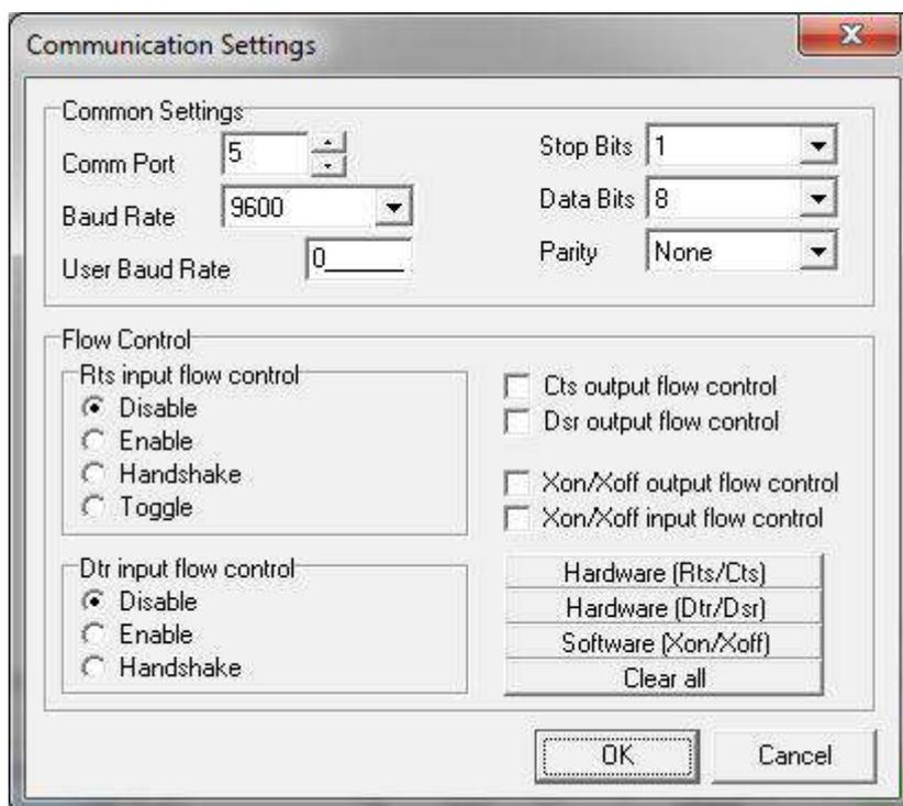
The above example shows the external Compass sensor on COM 3 which in this case is Port A on the MicronNav100 Hub and the external MRU (pitch/roll) on COM 5 which in this case is Port C on the MicronNav100 Hub. Check the integral sensor is switched off in Seanet Setup - Node 75 (MINIATTSEN) should no longer appear in the device list.
