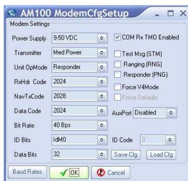
Change the Unit OpMode to Transponder, ID Bits to IdM 1-16, ID Code to 1 and disable the COM Rx TMO Enabled check-box (as shown below).
