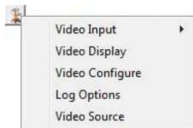
Video Input lists the video inputs (or capture devices) that are installed into Windows. These may include internal capture cards, external USB devices and built-in webcams (if using a laptop computer).
