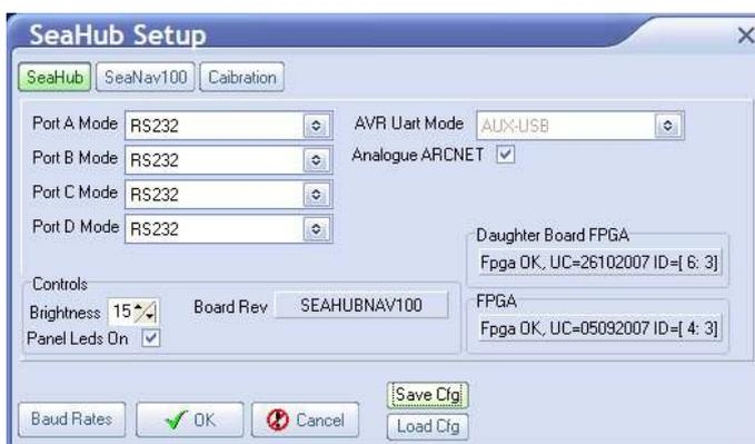
Confirm the settings and close the SeaHub Setup page. Apply power to the Micron Sonar/ROV and once the sonar has initialised the Main Setup page should list three Node numbers in the table - the MicronNav100 Hub (SEAHUBNAV100), the USBL Head (MINIATTSEN) and the Micron Sonar (MICRON).
