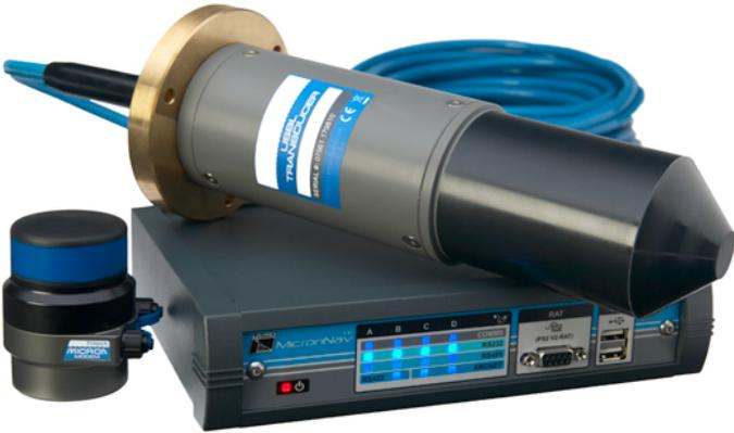
The system comprises a subsea MicronNav Transponder/Responder, a surface USBL transducer with integral magnetic compass and pitch/roll sensors, a surface MicronNav 100 interface hub and operating software under control of a host PC/laptop.
