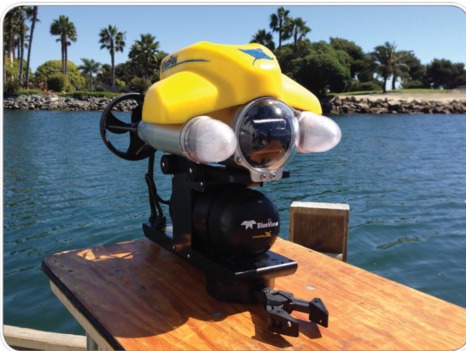
VideoRay Pro 4 ROV with V Series Imaging Sonar, Sonar Integration skid, Manipulator Arm
