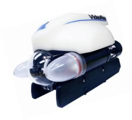
The **Explorer** ROV System is at the high end of entry level underwater Remotely Operated Vehicle systems. This simple and portable ROV system will give you eyes under the water down to 250 feet without getting wet.
