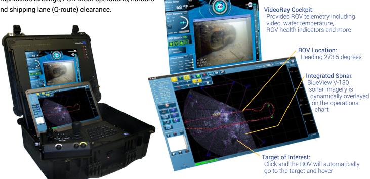
VideoRay RI CoPilot is Common Operator Interface (COIN) and SeeTrack™ compliant, allowing for the automated geodetic processing of AUV, SSS, diver, and GIS data to maneuver autonomously to predesignated underwater locations.
