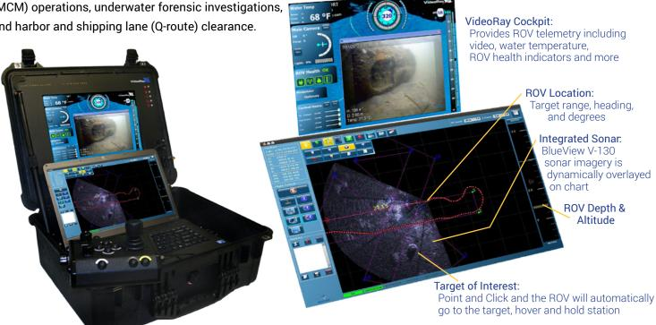
CPRI is Common Operator Interface (COIN) and SeeTrack  $^{\text{TM}}$  compliant, allowing for the automated geodetic processing of AUV, Side Scan, Tow Fish, diver, and GIS data to maneuver autonomously to predesignated underwater locations.
