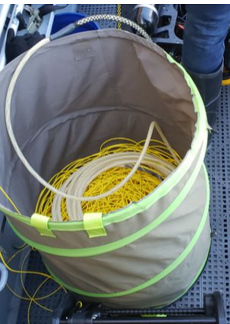
A tether bag made from a pop-up clothes hamper is another simple method of tether management on deck. Here, fiber tether has been loosely dropped in the bag. It will generally deploy easily without tangles or kinks.
