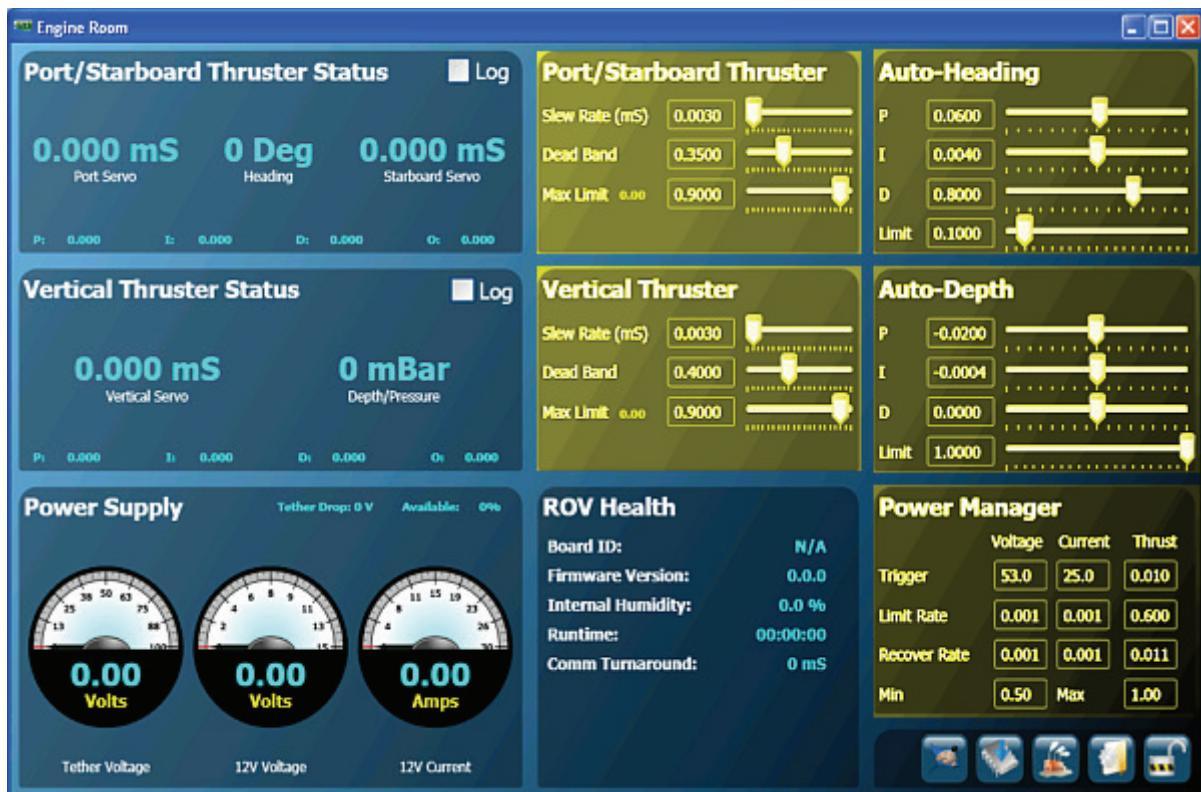
The systems tuning parameters are stored on the ROV. When you start VideoRay Cockpit, these settings are read from the ROV and the fields in the systems tuning windows are updated with these values. If no ROV is attached, the factory default settings are used.
