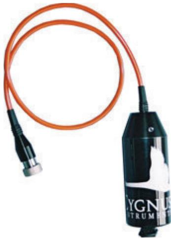
The Cygnus Instruments ultrasonic thickness gauge can be used to measure metal thickness even through coatings. The probe does not need to touch the surface under test, as measurements can be taken through 5 mm (0.2 inch) of water. Readings are not influenced by the probe orientation.
