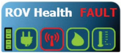
Sample ROV Health Instrument indicating a communications fault.
