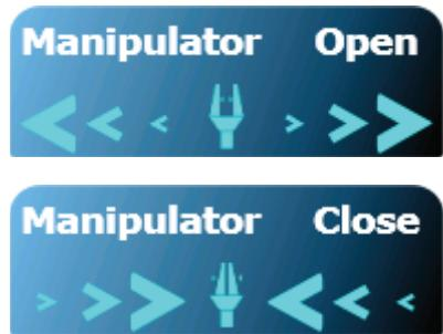
The size and display of the Manipulator Status Indicator can be adjusted. See the [Instruments](#) section of this guide for more information.
