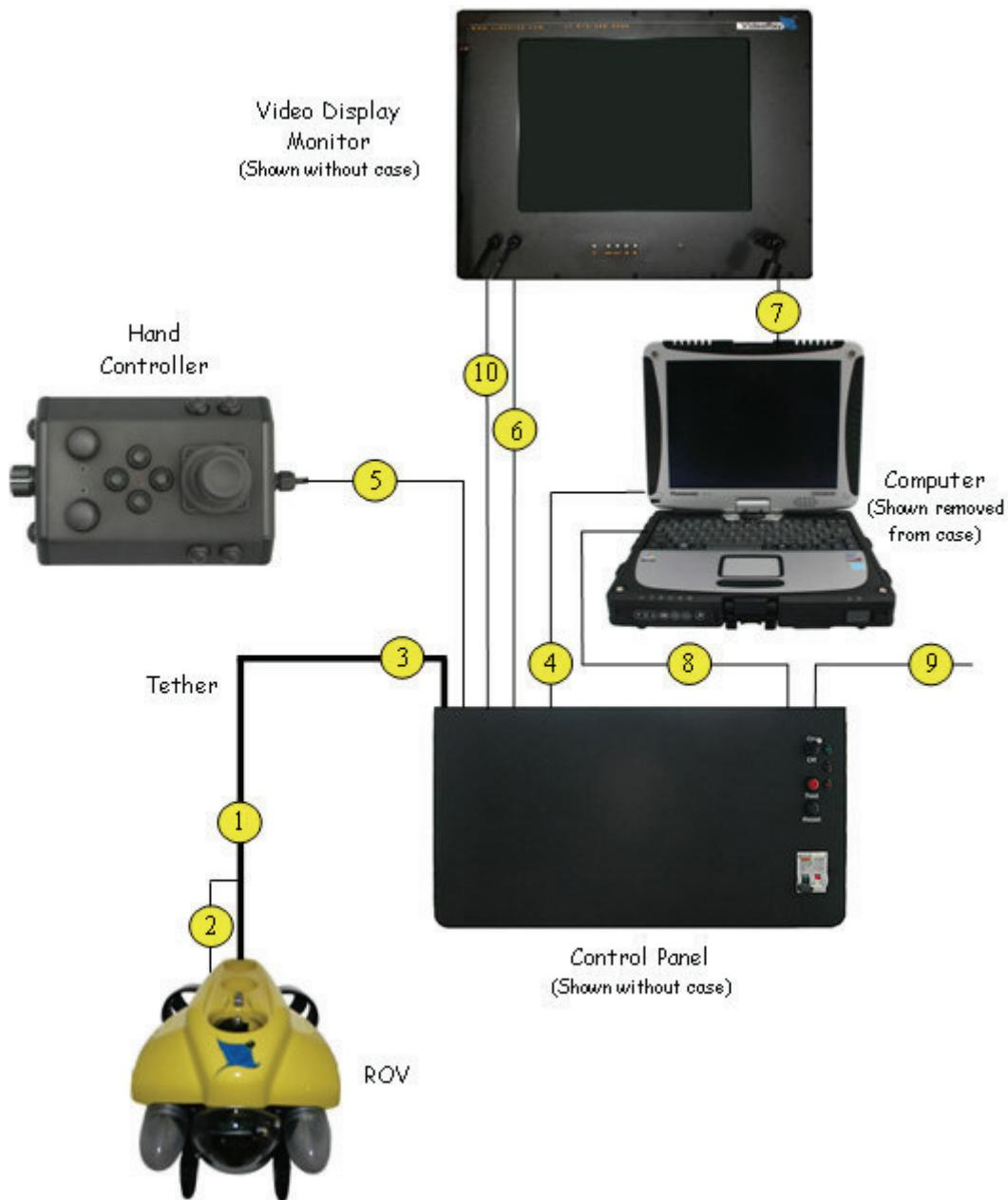
1. The male tether connector on the ROV is connected to the female connector on the tether.
