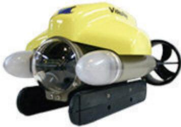
The Pro 4 ROV (Remotely Operated Vehicle) is depth rated to 300 meters (1000 feet).
