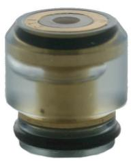
Cartridge seal with an acceptable bubble - this seal is okay to use.
