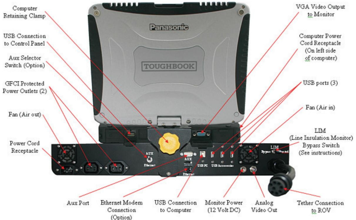
The control panel includes the following switches:
