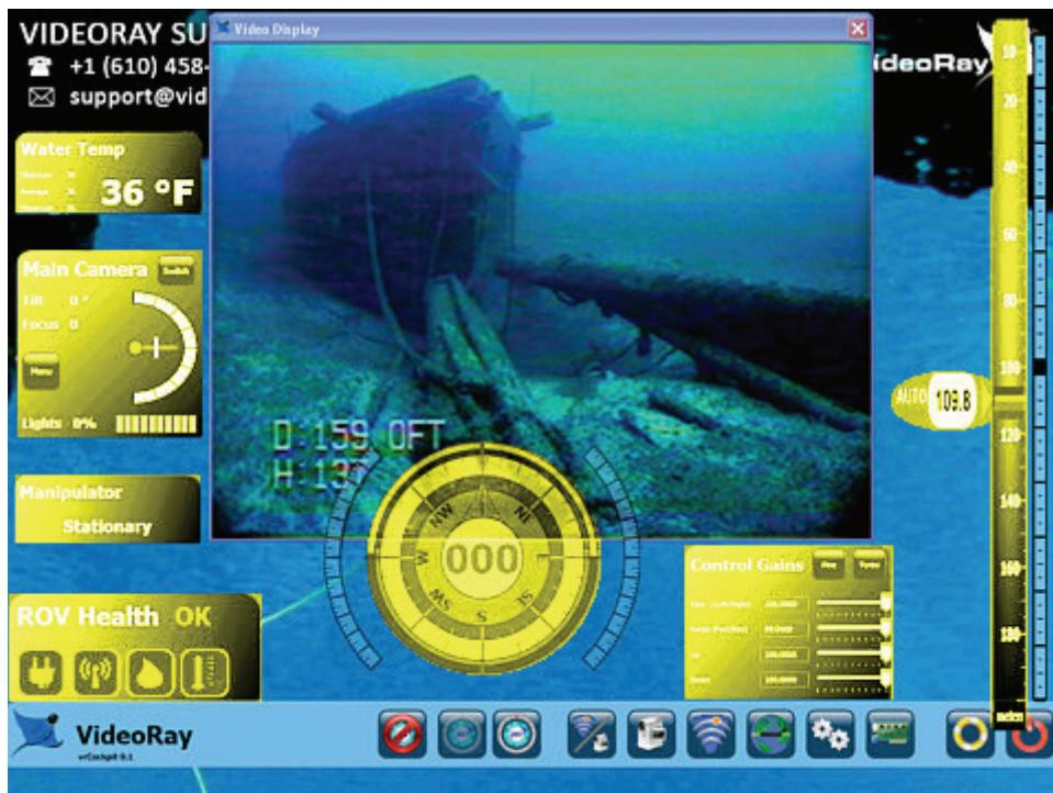
VideoRay Cockpit Instruments Highlighted in Yellow
