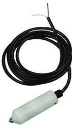
The Buckley's CP (Cathodic Protection) probe can be used to assess and monitor corrosion inhibiting systems. The probe mounts on the ROV. The probe is available in both contact and proximity versions. A calibration cell is also available.
