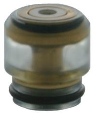
**CAUTION** Nearly empty cartridge seal - this seal should have been replaced when the oil level reached 1/2 of the original volume.
