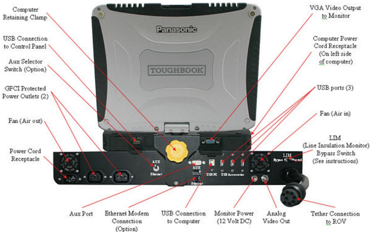
The control panel includes the following switches:
