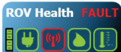
Sample ROV Health Instrument indicating a communications fault.
