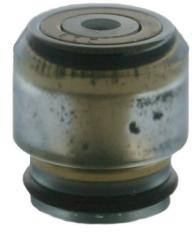
**CAUTION** Cartridge seal with contamination - this seal should be replaced.
