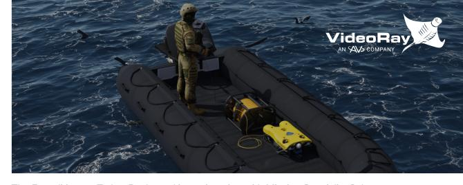
The Expeditionary Tether Reel, used in conjunction with Mission Specialist Subsea Vehicle Batteries, provides unmatched mobility and a small operational footprint without sacrificing performance or mission range. No topside power source is necessary when operating in this configuration, allowing for unlimited ROV deployment options.
