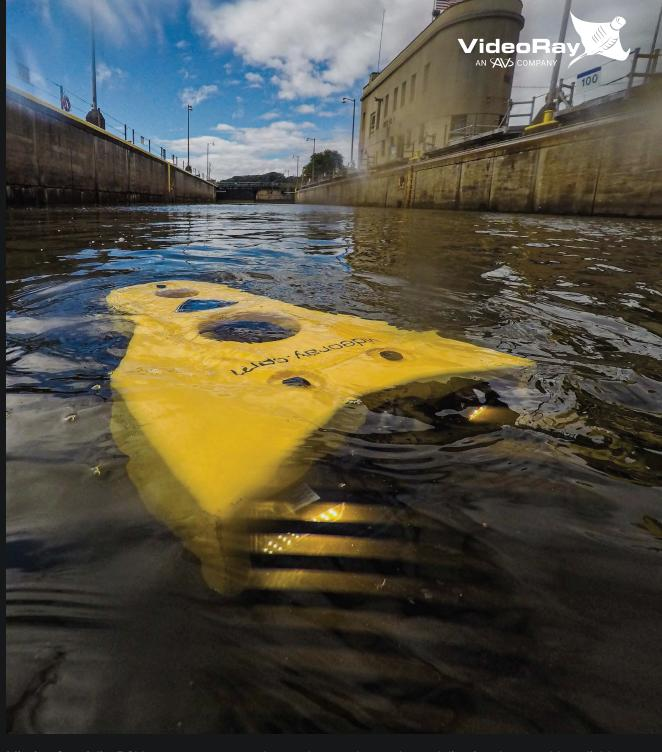
Mission Specialist ROV systems are rugged enough to work anywhere, delivering the portable, reliable systems you need to handle tough jobs in challenging environments. The Mission Specialist Pro 5 system is designed for optimal performance when size, speed, and efficiency matter most. Weighing in at 11.8 kg (26 lb), the three-thruster system has a forward speed of over 4.4 knots and a 300 meter depth rating.
